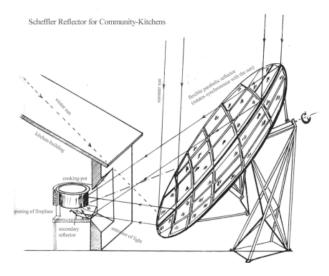
The building needs to have a north-facing wall, no large buildings or structures close to the dish, and sloping roof to allow the sun to shine on the dish during the daytime and throughout the year. The idea of the Scheffler Parabolic Cooker is basically quite simple in practice: it concentrates the solar radiation to one point through absorption onto the black coloured surface a cooking vessel, this concentrated energy is converted into heat and used to cook food inside the cooking vessel.
